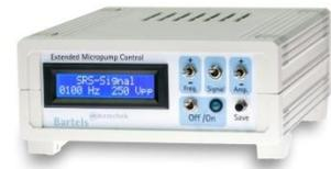
The mp6-OEM driving electronics is also capable to run the pump for gas applications, however there are some limits. With this driver the pump is specified to run between 85 - 270 Vpp of pump amplitude and 25 - 226 Hz of pump frequency. Higher frequencies are possible to achieve with additional circuitry, but the amplitude and signal quality degrade due to the limited energy conversion of the driving chip. So the overall performance of the driven pump will not increase linear anymore.
