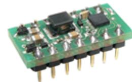
In comparison to the mp-x the mp6-OEM is weaker when pumping air; 11 ml/min and 50 mbar at 270 Vpp and 226 Hz. The evaluation kit mp6-EVA applies this controller.
