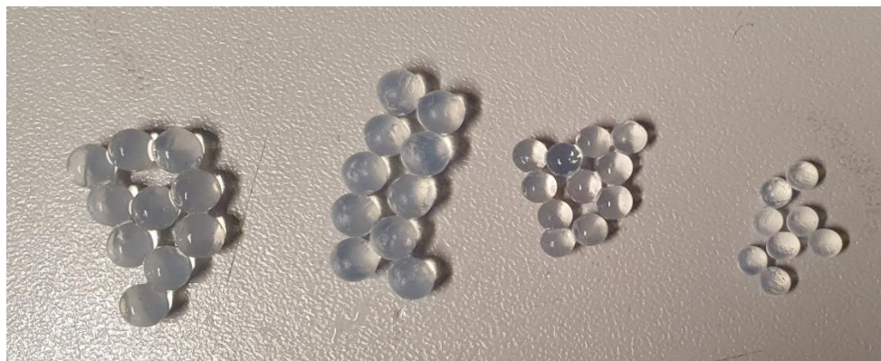
Figure 3 Generated Alginate beads; From left to right: 3.75 mm, 3 mm, 2.6 mm, 2.5 mm in diameter
