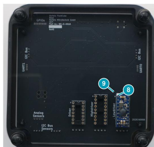
B Underside: mp-Lowdriver installed
