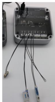
Figure 7. FluidCube | Switch connections, valve-driver orientation and example valve wiring.
